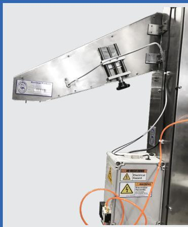
Air Blow system to eject wrong orientated caps
